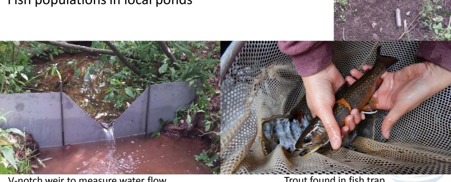
V-notch weir to measure water flow.
